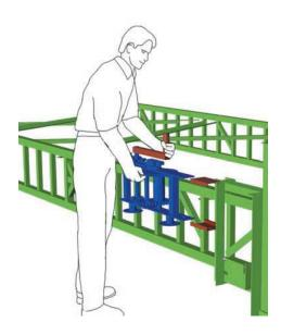
11. Slide the winch (handle side up) into the winch receiver and hand-tighten the bolt. Be sure to match left-hand winches to left-hand brackets and right-hand winches to right-hand brackets. Red markings indicate left-hand components. DO NOT crank the slack cable onto the winch now, that comes later.
