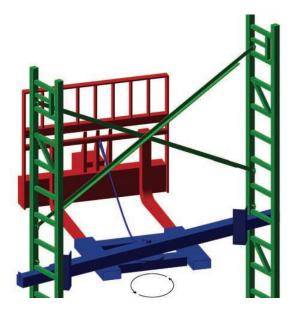
The tower can be swiveled 60° in either direction in order to land it parallel to the wall. This allows you to drive up to the wall from just about any angle, such as when turning corners, insets, inside corner returns, and other difficult job layouts.
