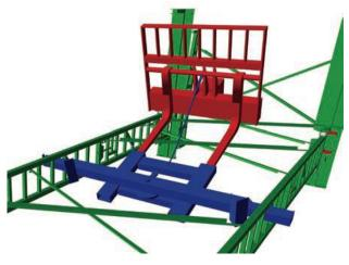
Releasing the rope will cause the plungers to extend under spring tension, capturing the towers on the swivel forklift bar. The towers may now be raised.
