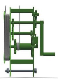
A flat spot will not reduce the load-carrying ability of the cable. In this application, a flat spot is only a dimensional, rather than a structural, imperfection. Replace a cable if it is flattened to less than one half of its original diameter, or if it contains three or more broken wires in any one strand. Use only genuine Non-Stop cables. Plain steel cable will corrode and is not OSHA-approved for this application.
