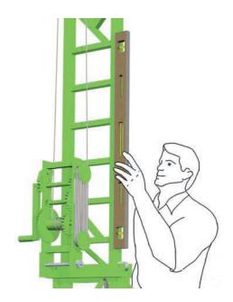
19. Plumb the tower. First plumb each individual leg, then raise the low leg of the pair by turning both leveling jacks an equal number of turns. Place your level on the tower itself to get true readings; never place it on the elevating bracket.
