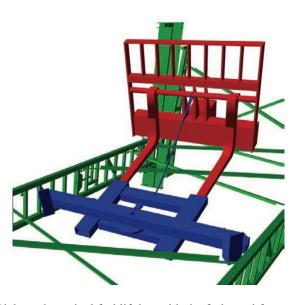
14. Pick up the swivel forklift bar with the forks and fasten the safety chain to the mast with a small amount of slack left in the chain. Pull the rope to retract the plungers on the swivel forklift bar. You can now position the bar between the towers. **Do Not Insert The Bar In A Space That Contains X-brace Locks!**
