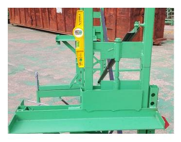
6. Plumb the tower. First plumb each individual leg, then raise the low leg of the pair by turning both leveling jacks an equal number of turns. Place your level on the tower itself to get true readings; never place it on the elevating bracket. A quality magnetic torpedo level is sufficient for plumbing.
