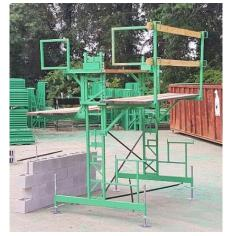
Climb up PAST the work platform a few feet, move around to the other side of the tower, and then step down on the work platform.
