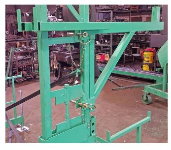
10. If you are using more than one extension, you will need a laborer's bracket. Some users like to employ two laborers brackets to a tower to make it easier to hop plank.
