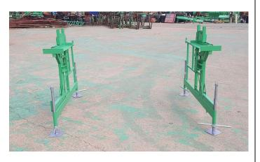
1. Stand up a right- and left-hand (left indicated by red paint) stub base tower with carriage about 7 feet apart. Make sure you are on a firm foundation according to OSHA standards. Use base plates or leveling jacks as required.
