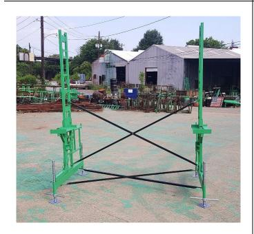
3. Connect the two towers using x-braces as shown. Be sure that the "V" of the angle iron faces downward, toward the bottom of the base tower. This will keep mortar droppings from collecting on the brace.
