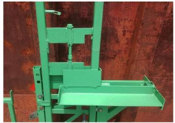
2. Insert a 4'3" extension into the stub base tower and tighten the bolt with a 15/16" wrench. DO NOT use an impact driver to tighten the nut as damage can occur. If you happen to insert an extension backwards, the bolt will be 1" off center and your x-brace locks will be on the wrong side.
