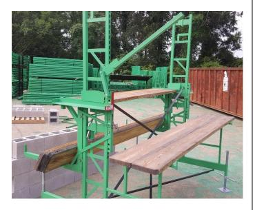
9. To jack the tower, insert the jack handle into one of the four holes shown and push downward. Do not jack one leg more than 6 notches out of level with the one beside it. You may use the same jack handle to jack any leg. We recommend that you jack every 5 courses of brick and 2 courses of block to keep the wall waist high to the mason. If you find the jack handle is obstructed by an x-brace, change it to another hole.
