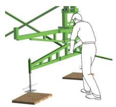
11. Before landing the tower at the wall, attach it to the tower beside it with a straight brace (this will set your 7 foot spacing automatically). As you lower the tower, one leveling jack will make complete, weight-bearing contact with the ground before the other three. When it does, stop lowering and tighten the other three jacks. The tower will be almost plumb.
