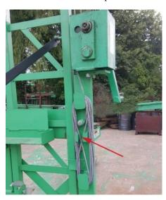
carrying ability. In this application, a flat spot is only a dimensional, rather than a structural, imperfection. Replace a cable if it is flattened to less than one half of its original diameter, or if it contains three or more broken wires in any one strand. Use only genuine Non-Stop cables. Plain steel cable will corrode and is not OSHA-approved for this application.
