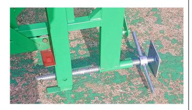
7. If you are going to manually lift the tower, add the leveling jacks and fasten them in place with the provided snap pins and skip to Step 10. If you will be lifting the tower with a forklift, this step will come later.
