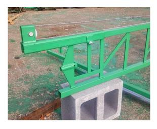
6. Mount the pulley on the tower as high as possible. Be sure the cable is not twisted at any point between the winch and the pulley. Do NOT crank the slack cable onto the winch now, that will come later.
