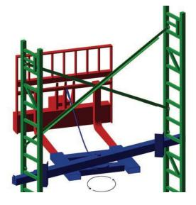
The tower can be swiveled 60° in either direction in order to land it parallel to the wall. This allows you to drive up to the wall from just about any angle, such as when turning corners, insets, inside corner returns, and other difficult job layouts.
