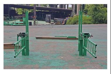
1. Stand a right- and left-hand (left is indicated by red markings) base tower with carriage on edge about 7 feet apart.
