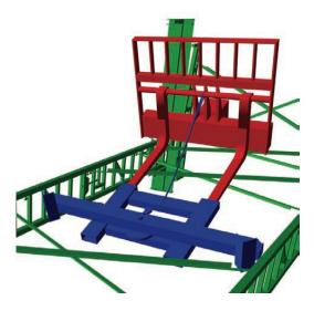
8. Pick up the swivel forklift bar with the forks and fasten the safety chain to the mast with a small amount of slack left in the chain. Pull the rope to retract the plungers on the swivel forklift bar. You can now position the bar between the towers
