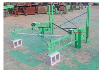
2. Attach the base towers together using 3 x-braces installed as shown. Be sure that the "V" of the angle iron faces downward, toward the bottom of the base tower. This will keep mortar droppings from collecting on the brace. Put a 12" block, or something similar, under the end of each tower. This will make it easier to add extensions to the tower.
