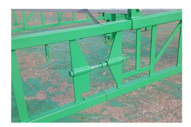
3. Insert 4'-6" extensions and tighten the bolt snugly with a 15/16" wrench. DO NOT use an impact driver to tighten the nut as damage can occur. If you happen to insert an extension backwards, the bolt will be 1" off center and your x-brace locks will be on the wrong side.
