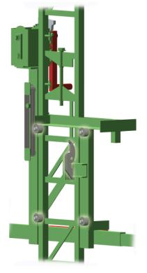
**Safety Assured**Standard Duty uses an automatic inertial safety device that cannot be defeated and is unaffected by mortar and debris. In the event of a cable failure, the safety will prohibit the carriage from free falling and since it is completely passive, it does not need to be disengaged or reset.
