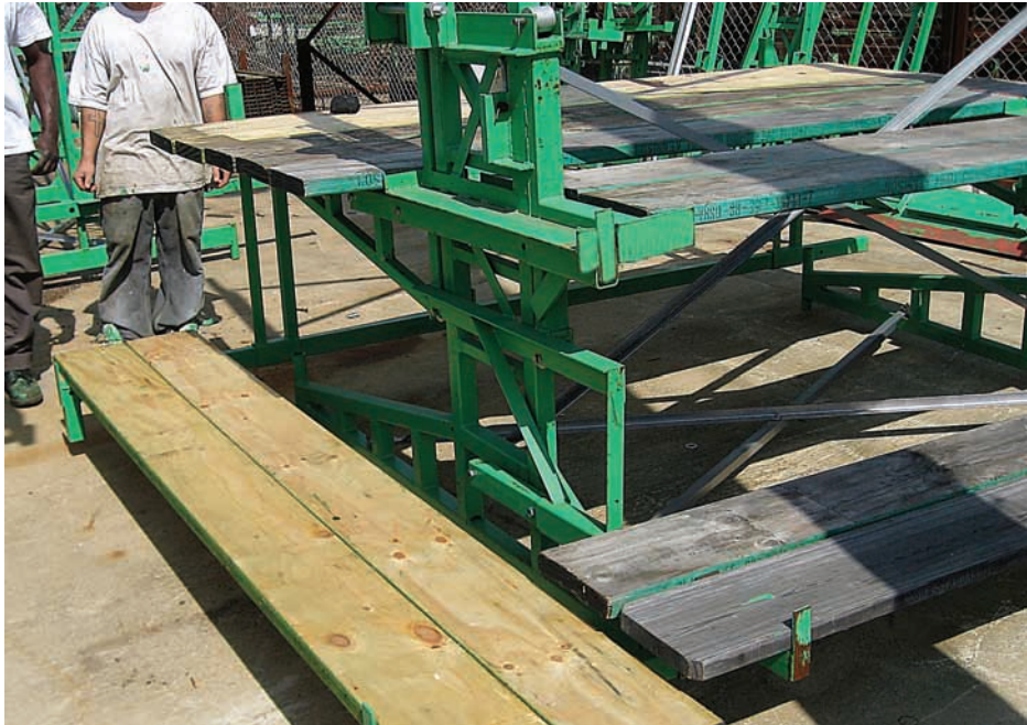
Photo 2: The Corner Brackets support one to three planks (the new boards) on either, or both sides of a tower, simplifying the layout of inside corners.
