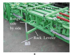
1. Put the rack leveler with two leveling jacks in the middle of your work area. Spin the jacks up until the top of the bar is about 13-1/2 inches above the ground.
