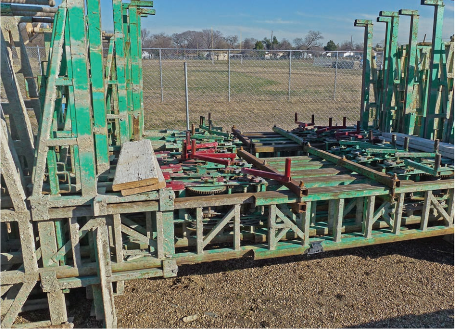
Photo 5 - This contractor clamps his base towers together in packages of 10. Each one is four feet wide, allowing him to put two packs across his trailer. Each pack is 14 feet long.
