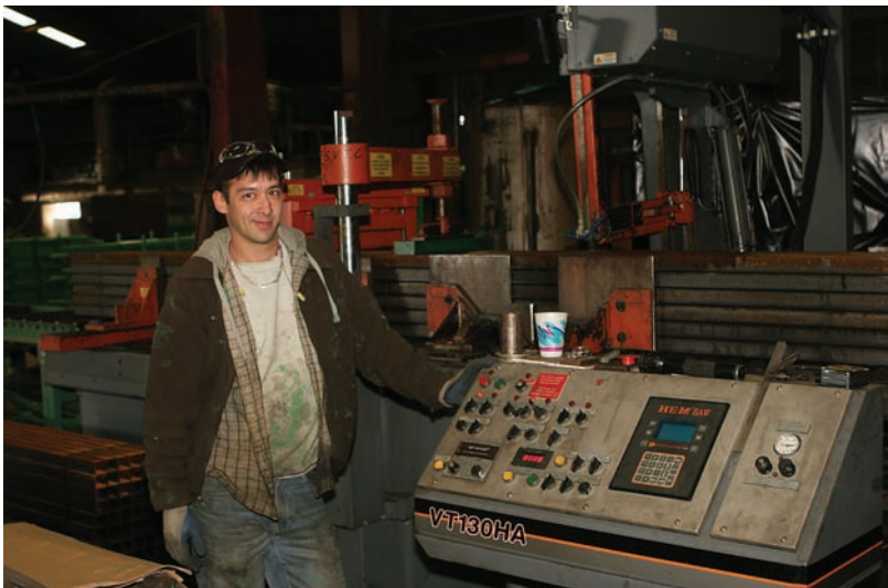
Non-Stop uses computerized saws for exact cuts on raw materials.
