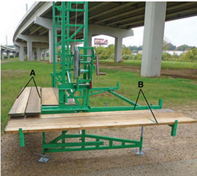
Photo 5 - The Inside Corner Arm can be adjusted for 0 to 5 planks (area "B").
