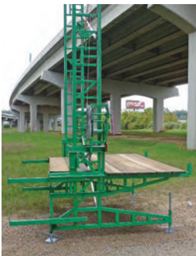
Photo 3 - Flexible planking is standard. The top and bottom masons outriggers adjust for 0 to 5 boards to fill the inside of an elevator shaft.
